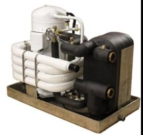
Equipped with industry proven high efficiency low starting torque scroll compressors with CPVC safe PVE oil. Stainless steel plate evaporators with multiple safeties including low pressure control, flow switches, and mechanical freeze protection preventing freeze conditions.
